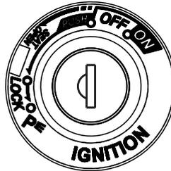
The main switch/steering lock controls the ignition and lighting systems, and is used to lock the steering.
