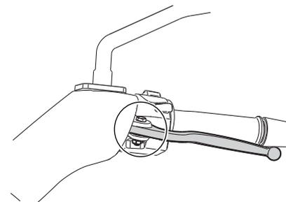
The pivoting points of the front and rear brake levers must be lubricated
