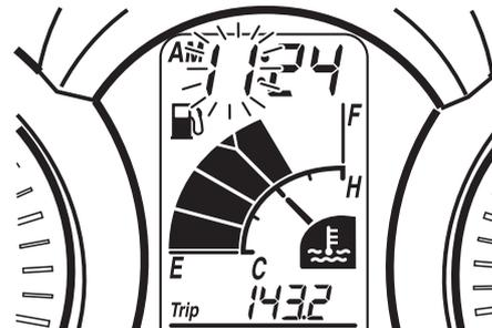
3. Push the “SELECT” button, and the minute digits will start flashing.
