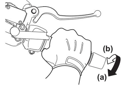
The speed can be adjusted by opening and closing the throttle. To increase the speed, turn the throttle grip in direction (a). To reduce the speed, turn the throttle grip in direction (b).
